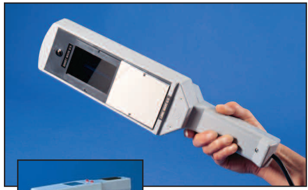
Handheld UV Lamps are lightweight 6-watt models.
